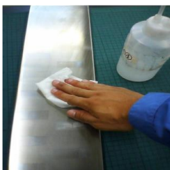
1. Use cleaning solvent to remove contaminants like dust, rust, oil, etc.
